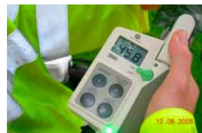
A Minolta chlorophyll meter SPAD 502 measuring the chlorophyll content of leaves in the field.
